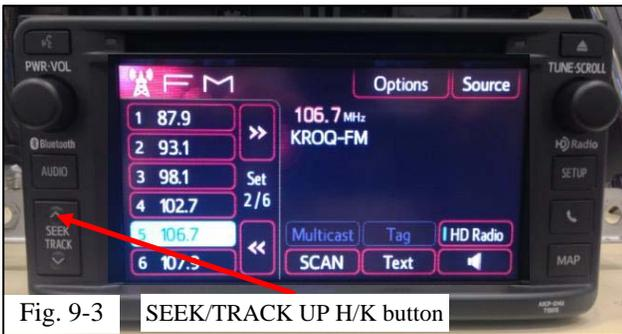
(c) Press the SEEK/TRACK Up H/K button (Fig. 9-3). Confirm that the radio tunes to a FM radio station and sound is heard.
